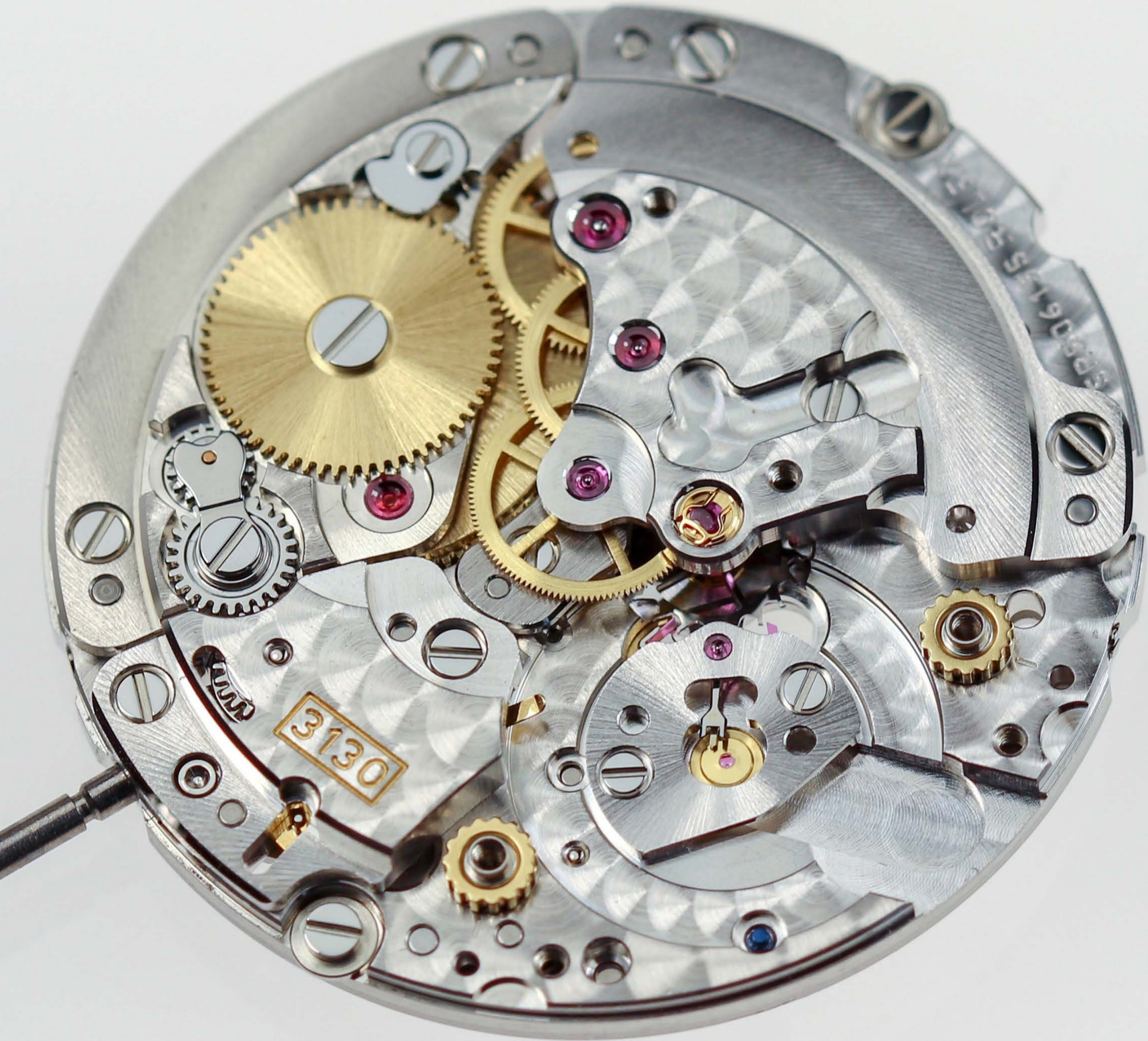
The balance assembly removed showing the Swiss lever escapement.
